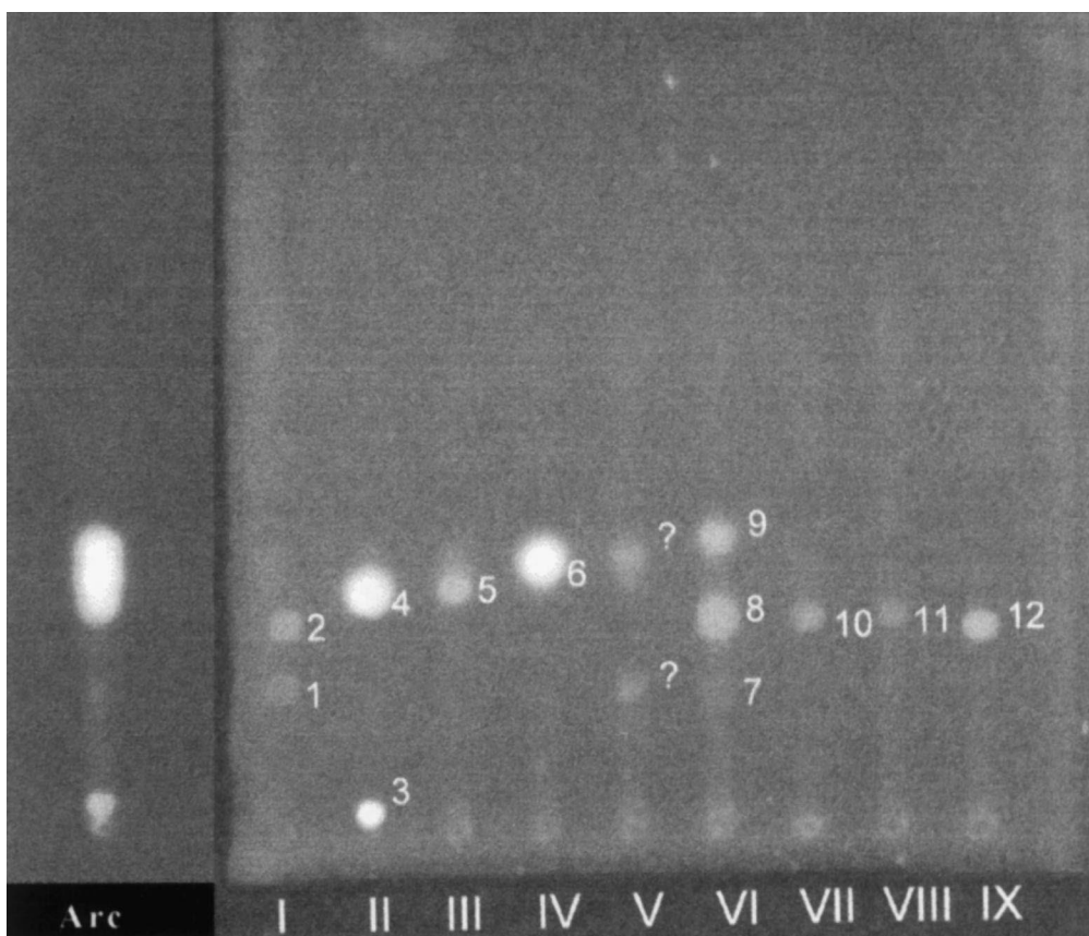
Fig. 5. The Camag Reprostar 3 photography of TLC plate with applied fractions collected during HPLC separation and Archangelica off. Extract scanned in black and white mode. Number of substances as in Table 1, ?: unidentified substances. Arc: Archangelica officinalis extract. Roman numbers of fraction as in Fig. 3.
